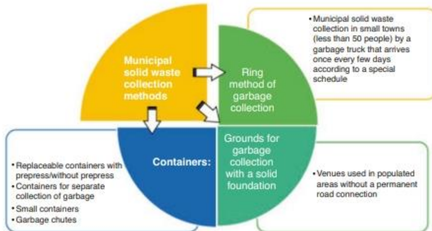
Fig. i Principal techniques for collecting municipal solid trash from the populace and infrastructure. Source: (Scarlat, Dallemand, Monforti-ferrario, & Nita, 2020).
